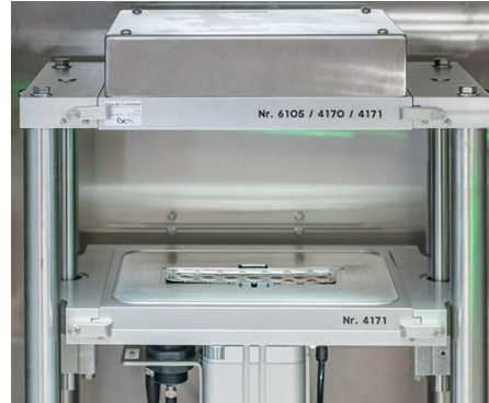
Test chamber with the format part to test blister packages
